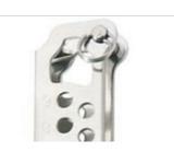
Some years latter, we accepted the device with a screw and a bolt instead of pins. What we usually refer as a "sta master" adjuster, even when there is several brands in the market. This device was much more safe. The shrouds are never free during the adjustment, and it allows a sailor to adjust the length of the shroud releasing the tension of the rig and manual turning the screw.
