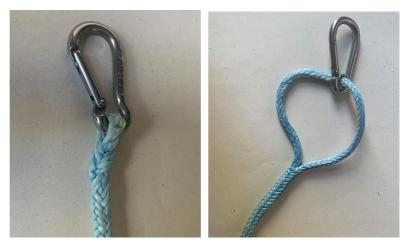
The proposal contains also a minimal diameter on line. The reason for this is because smaller lines might break. If a capsize happens downwind there is not much problem, but when it happens upwind with the centerboard down, when the boat is turned upside down the centerboard will move and has plenty of distance to get momentum. If the line is not strong enough it will cut. I would also recommend only dyneema type lines or at least with a dyneema core.
