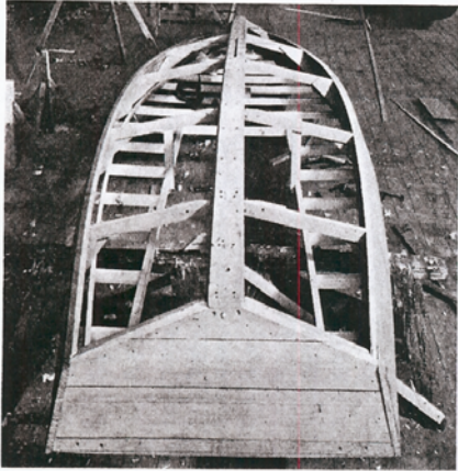
23—This shows hull ready for bottom planking
