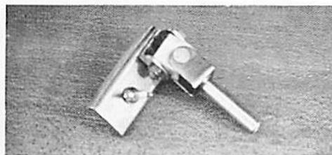
The gooseneck is all stainless steel. It is much stronger than the old aluminum one. Also it will not freeze up when used in salt air.
