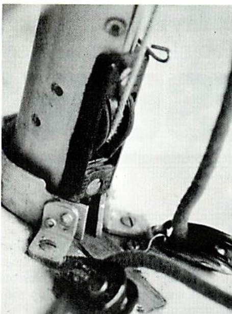
Fig. 1: A slightly different arrangement. Note that the retention collar is screwed to the liner. (Dan Williams photos)
