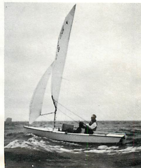
Craig Leweck, again, with properly eased jib halyard and vang. Note the upper batten is set parallel to the boom with correct vang trim.
