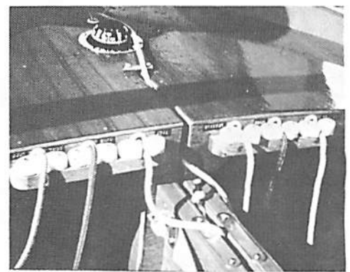
Each cleat has a sign which tells you what line you are pulling. Lou Varalyay's idea.
