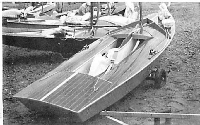
New Fiberglass Hull with Wooden Deck and Alloy Spars made by Olympic Boats of London. Note pivot centerboard.
