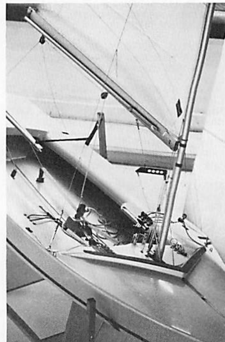
Sylvie's Skipper Snipe with whisker pole on the boom, and cockpit controls within easy reach.
