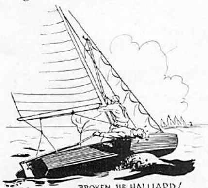
BROKEN JIB HALLIARD! ED McHENRY USES SPINAKER POLE AND SPARE TILLER TO HOLD JIB UP
