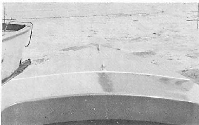
Fiberglass paste cleaner can be very effective in restoring a chalked or faded surface as indicated by glossy area which has received treatment. A substantial coat of protective wax will maintain the finish
