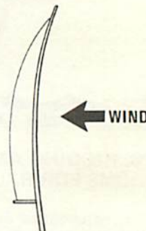
7. When mast bows to leeward sail twist is reduced.
