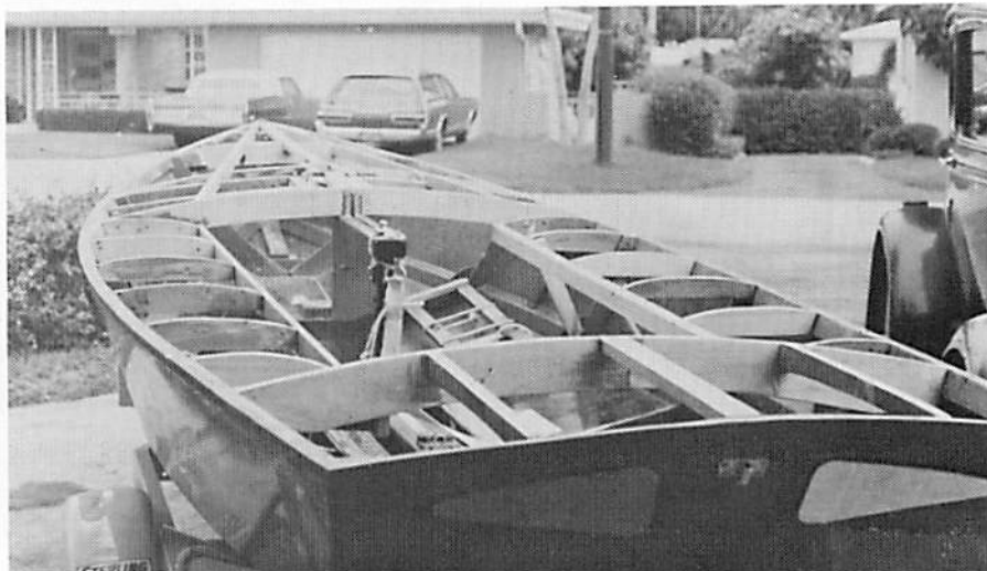
7 - Completely reframed in spruce and cedar. I used Harold Gilreath's curvature for fore and after deck, but increased roll of side decks.
