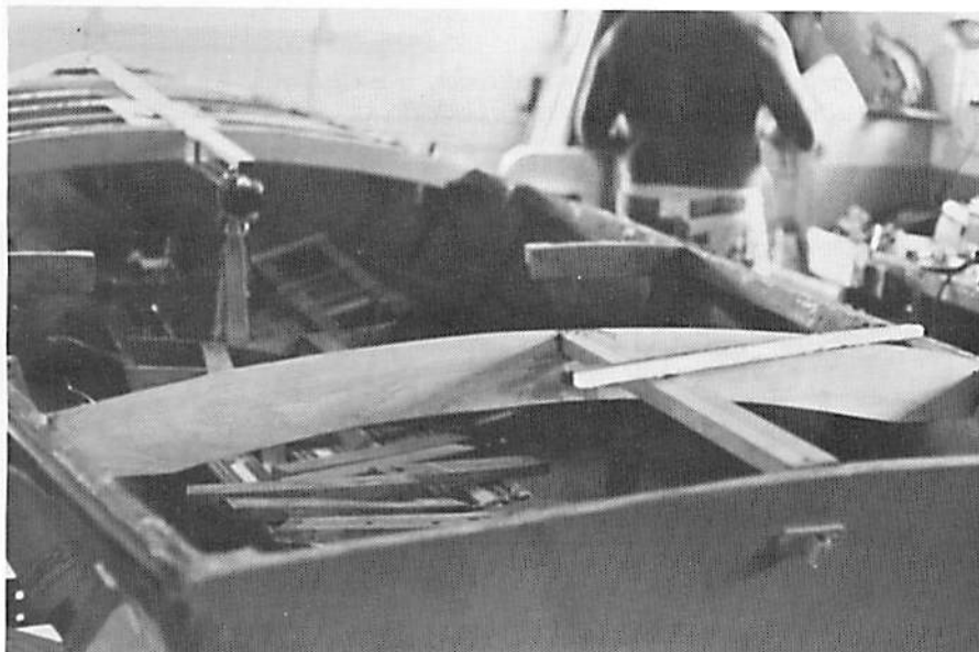
4 - Cockpit frames were immediately replaced, so as not to lose hullshape
