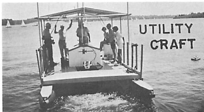
This general utility pontoon boat (or raft) patrols the course during races on Lake Cowan, Ohio, home of Fleet 443. Used mainly for rescuing disabled craft, it has an unique and efficient feature of a wide notch cut into the stern. The bow of the boat
