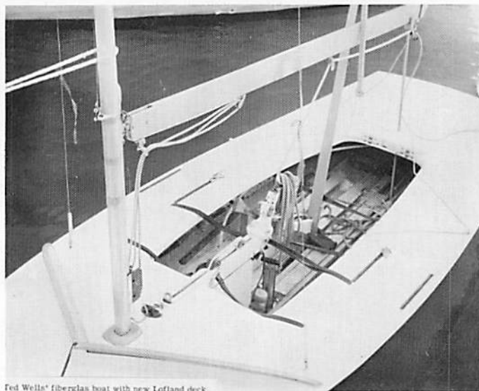
Fed Wells' fiberglass boat with new Lofland deck.
