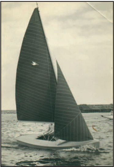
Below: an early Snipe with jib sheets led outside the shrouds.
