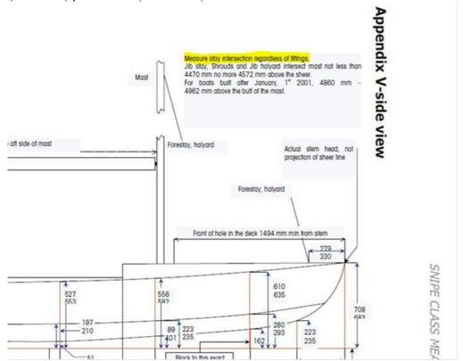
The picture is an excerpt of Appendix V-side view in which is highlighted in yellow the way finding the intersection point of the stay with the deck.
