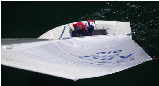
Using our Advanced Sail Analyzer software, we can get a really good look at the differences in flying shapes from these two photos comparing mainsheet tension differences. The software is used to analyze the flying shapes of the photos and yields Max Camber, Draft position, Twist, Entry and Exit angles, Forward and Aft shaping. The software also creates a 3D IGES file for each photograph to provide a 3D overlay comparison view from any angle.
