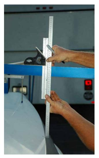
Chine widths [horizontal measurements] are found measuring with the large caliper the distance between the marks [see Station Measurements] at each station. The slider shall be beetween the correspondents marks on the large caliper.
