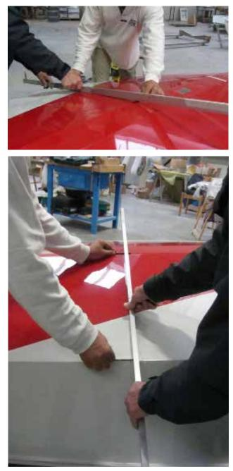
The hull measurements are now complete and the boat is ready turn right side up. Before you do so check to be sure that you have the Hull Datum Point mark and the sheer line marks for each station on the deck.
