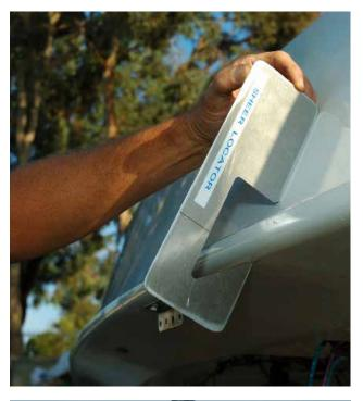
Make a pencil mark at this point now pivot the tool so that it is parallel to the locator tool which should be hanging 90° to the cross member. See photo. (needless to say this is tricky at first).
