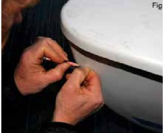
If the edges of the tool don't touch the surface, the radius is correct; if the edges of the tool touch the surface and there is space in the middle, the radius is greater than allowed; if the tool fits the curve the radius is the maximum allowed. See Fig. 3 to 7.
