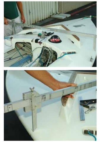
Now measure the width of the cockpit from the inside edge of the deck on the port side to the inside edge on the starboard side, this distance shall be no more than 1016mm. If the deck curves down with a radius, to find the measurement point place the large calipher on the sheer lines at the maximum width of the cockpit, measure down the distance from the top of the bar to the sheer line, add 51mm. The cockpit width shall be measured at this exact height.
