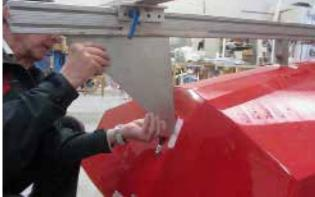
The sheer and chine depth at the transom can be measured by either the process used for the stations or simply measuring down to the drawn lines with a high quality rule.
