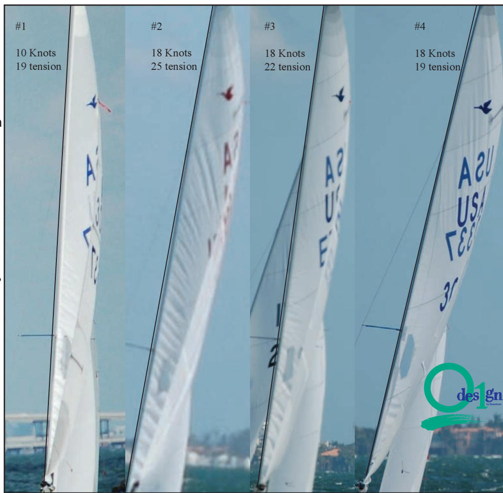
Photo #1: Same tension on #4, but too tight for lighter air
